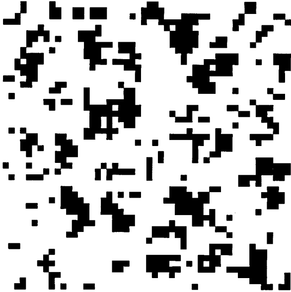
FIG. 1. Snapshot of a population of interacting particles that represents an evolving, two-phase microstructure. This 625-particle configuration on a 50 \times 50 grid produces the normalized information entropy H'(m) curve calculated at time t = 1000 in Fig. 4.
